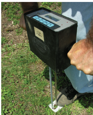
Fig. 1. Measurement of soil depression by penetrometer P-BDH 3A.
